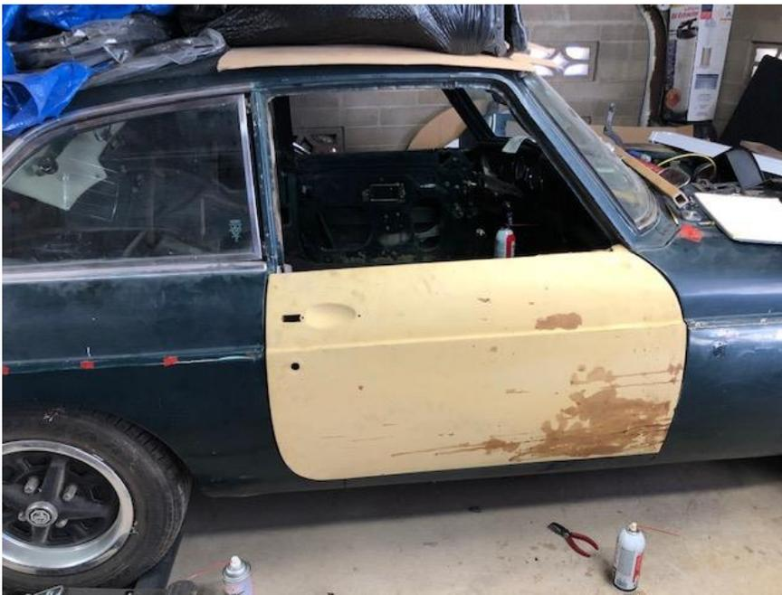
The final picture shows the door in place & closed. The vent window fits properly and with some fitting and fettling the gaps should be pretty good.
