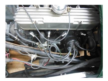
This month I updated all the fuel lines from the tank to the carbs, cleaned and sized most of the jets, removed carb and in-line fuel filters for cleaning or replacing and redid all the primary circuit wiring. Plugs were cleaned/re-gapped, points cleaned and reset and timing adjusted. The oil change was done last fall, so I passed on that and simply replaced coolant. With the help of #1 mechanic Megan, brakes and clutch hydraulics were bled and the car road tested.
